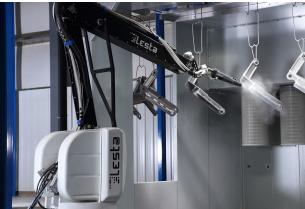
With Lesta Self-Learning Robots, a manufacturer no longer needs to shut down the entire finishing line every time a program needs to be created to paint a new part. With user-friendly controls, adjustments can be made to fan, atomization, flow, and path speed to adapt to variables that could affect the application program.
